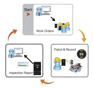
The Guardwatch will provide a mobile communications facility by NFC-enabled devices, this technique enables technicians to download up-to-date work orders from assignment, and to upload mission reports/records back to TPMS when he/she accomplish their mission.
