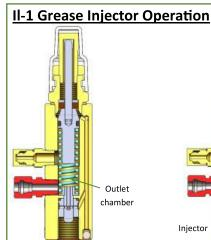
Stage 1 Grease injector is relaxed. Pump is not running, lubricant is not under pressure. The outlet chamber is full of grease from the previous cycle.
