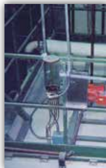
Gravity feed oiler on drying machine
