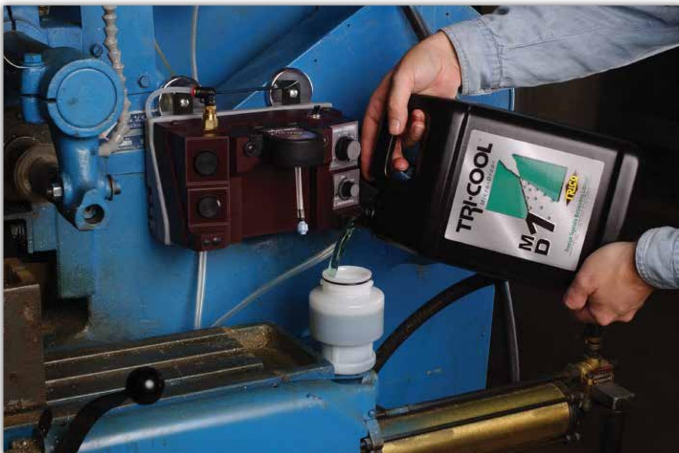
Micro-dispenser being filled with Tri-Cool MD-1 lubricant
