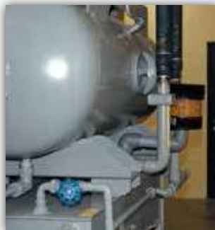
Watchdog Breather installed on a hydraulic reservoir
